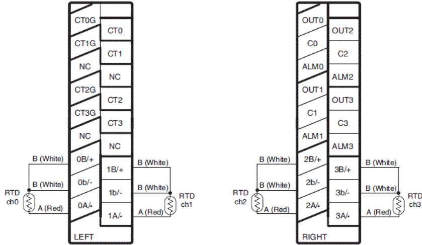
\* Colors in parentheses ( ) are the wiring colors (color of Y terminal) for RTDs made by Keyence Corporation.
