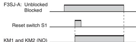
**Note:** Output turns ON with the rising edge of reset switch S1, but will not operate if there is a short breakdown in S1.
