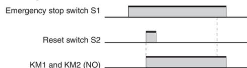
**Note:** Output turns ON with the rising edge of reset switch S2, but will not operate if there is a short breakdown in S2.
