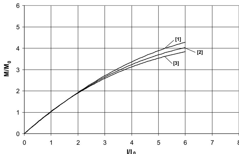
Torque-current characteristic curve CMP63S/
