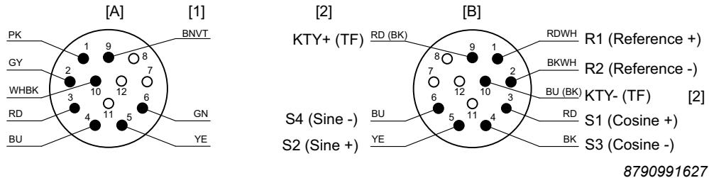
*Pin assignment of plug connector lower part*
